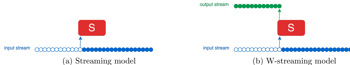
Figure 1.2: A comparison of a regular streaming model, and a W-streaming model. In (a), the output fits inside the memory. Therefore, the machine might store the output and report it in the end. However, the size of output in (b) is much larger than the size of memory. Thus, the machine needs to output respectively as soon as an input entry arrives (or at least output in small buffers).
