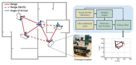
Figure 1: Overview of our 3D localization system for AR/VR. between nodes during two-way ranging can be used to estimate the angles between nodes. This adds an additional layer of constraint to the topology without needing extra measurements. We carefully select key edges to measure which maximizes the constraints in the topology and minimizes the latency.
