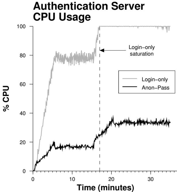
Fig. 4. The CPU usage on the authentication server measured every 5 seconds. The average CPU utilization for Login-only during the first stable segment (6,000 clients) is 77.9% ( $\pm 2.42$ ) and reaches saturation at about the 17 minute mark, or approximately 8,100 clients. The CPU utilization for Anon-Pass is 16.8% ( $\pm 0.73$ ) at 6,000 clients, and 33.4% ( $\pm 0.96$ ) at 12,000 clients (the second stable segment).
