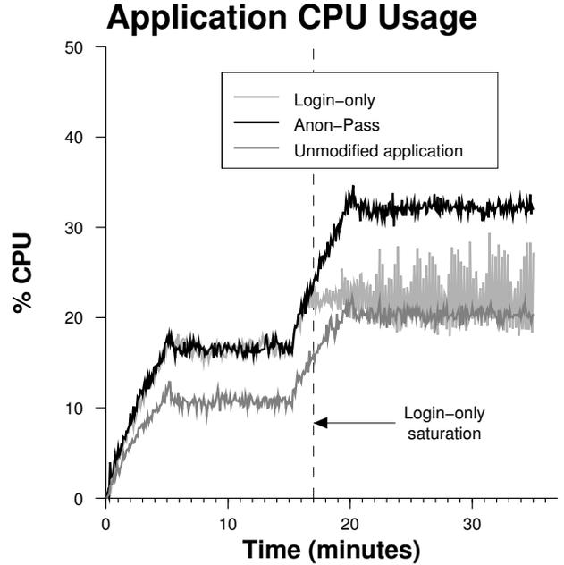
Fig. 3. The CPU usage on the application server measured every 5 seconds. The CPU usage with login-only follows the Anon-Pass behavior until the authentication server reaches saturation. Clients timeout and the application server has an overall drop in CPU utilization due to the lower number of clients successfully completing requests.
