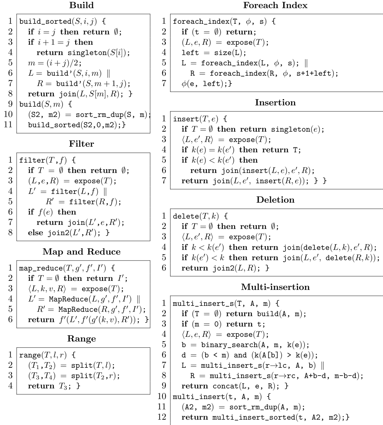
Figure 31: Pseudocode of some join -based functions – They are all independent of balancing schemes. The syntax S_1 || S_2 means that the two statements S_1 and S_2 can be run in parallel based on any fork-join parallelism.
