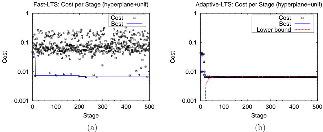
Fig. 11: LTS cost versus stage number for the HYPERPLANE+UNIFORM distribution ( $d = 2$ ,  $h = 0.1$ ) for (a): Fast-LTS and (b): Adaptive-LTS.
