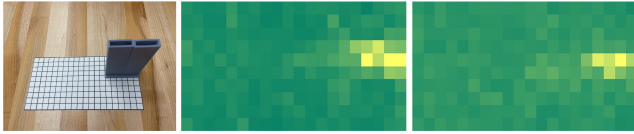
Figure 20: Scene reconstruction results at 1cm and 0.5cm resolutions. We modify the number of columns in the channel matrix to have a higher resolution.
