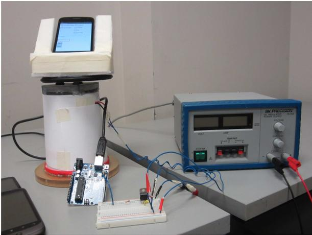
Fig. 16: Smartphone with external motor for rotation.
