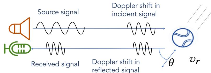
The magnitude of the frequency shift depends on the velocity of sound, the velocity of reflector object and the radial angle ( $\theta$ ).
