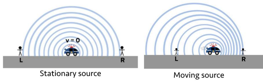
The frequency observed depends on the relative velocity between the source and receiver.
