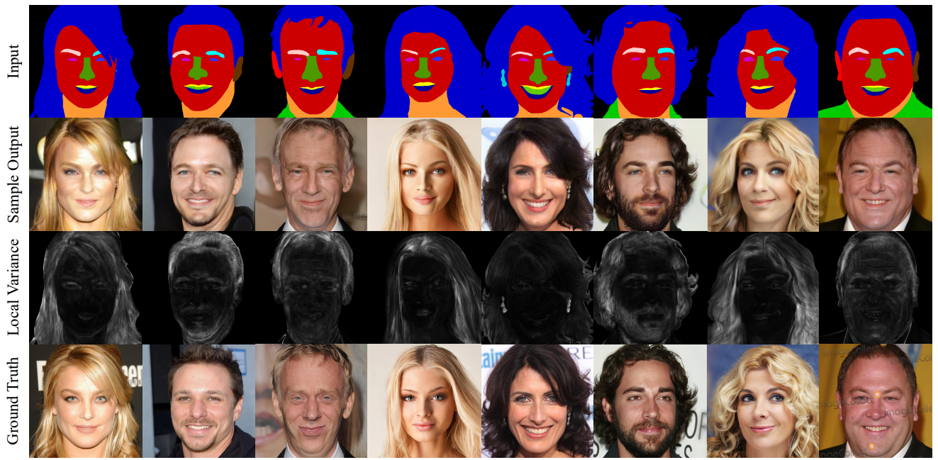
Figure 1. Examples of local stochastic variations. Top to bottom rows represent the input image, one sample output, the standard deviation of each pixel over 20 different outputs of the same input, and the ground truth image respectively.
