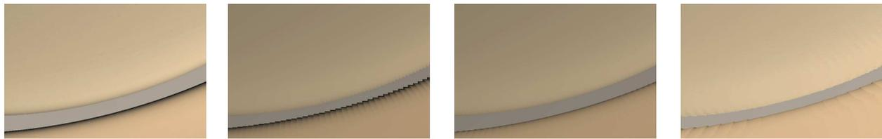
(a) Differential Points (157K pts.)      (b) Square Primitive (1037K pts.)      (c) Rectangle Primitive (819K pts.)      (d) Elliptical Primitive (180K pts.)
