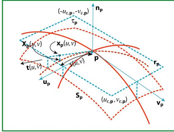
Fig. 3. Tangent plane parameterization of a Differential Point: The tangent plane  $\tau_p$  is parameterized by the  $(u, v)$  coordinates.  $S_p$  uses the same parameterization which relates it to  $\tau_p$  under the projection  $\mathcal{P}_p$ .  $u_{\epsilon, p}$  is defined by the constraint  $\|\mathbf{X}_p(u, 0) - \mathbf{x}_p(u, 0)\| \leq \frac{\epsilon}{\|\lambda_{u_p}\|}$ .
