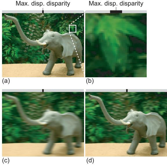
**Figure 11:** Comparison of aliasing, conservative filtering of individual views, and linear filtering in ray space. (a) Simulated view with aliasing apparent as ghosting artifacts, shown in close-up (b). (c) Simulated view with conservative filtering, (d) with ray-space filtering. Note how our approach preserves spatial frequencies on the zero-disparity plane.
