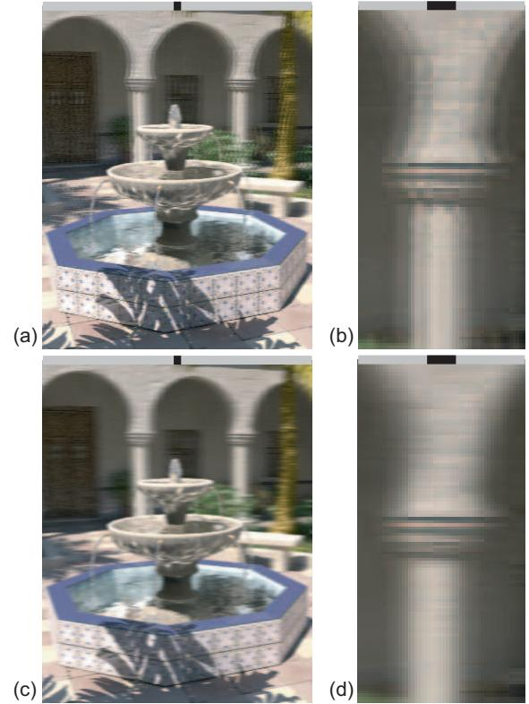
**Figure 12:** (a) Simulated view showing reconstruction aliasing, (b) close-up of ghosting artifacts; (c) using the combined resampling filter, (d) close-up reveals no ghosting problems. The black bar at the top of the images indicates the maximum display disparity.
