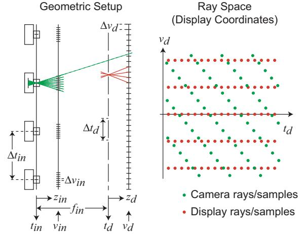
**Figure 4:** Mapping the input rays to display coordinates: Geometric setup (left) and sampling grids in ray space (right). The acquisition parameterization is translated by a distance  $f_{in}$  compared to the display, which corresponds to a shear in ray space. Each ray on the left corresponds to one sample point on the right.
