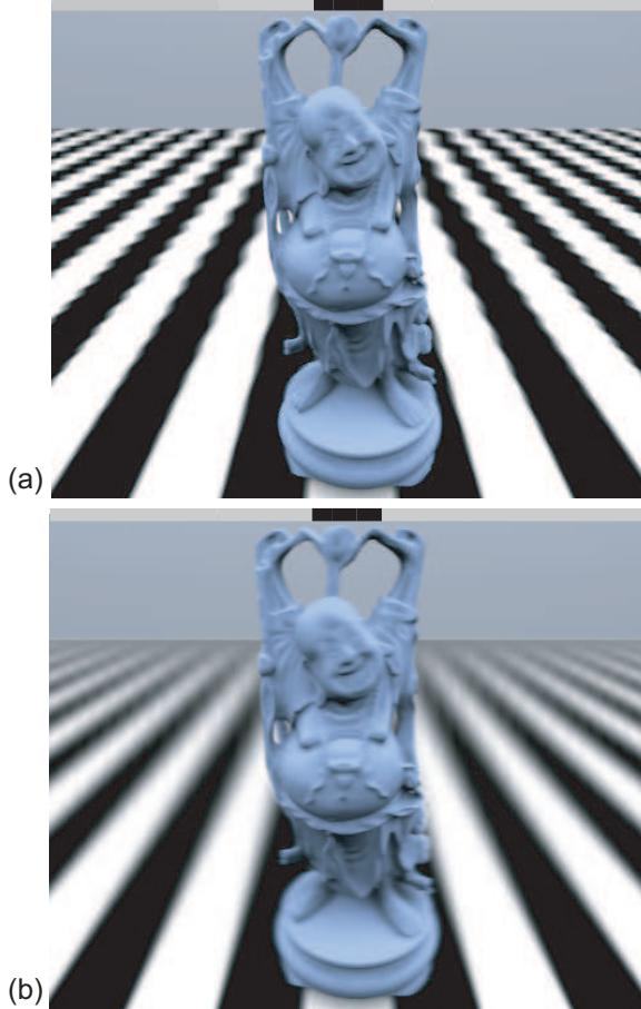
**Figure 6:** Resampling results: (a) Simulated view using only the reconstruction filter. This leads to pre-aliasing. (b) The combined resampling filter eliminates pre-aliasing. The black bar at the top of the images indicates the maximum display disparity.
