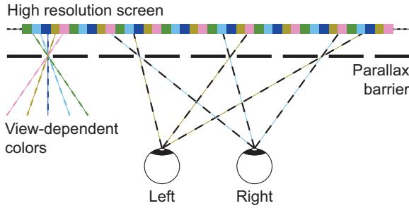
**Figure 1:** An automultiscopic parallax barrier display with five view-dependent subpixels per multiview pixel. We distinguish automultiscopic displays with multiple view-dependent subpixels from autostereoscopic displays that project exactly two views, one for each eye.
