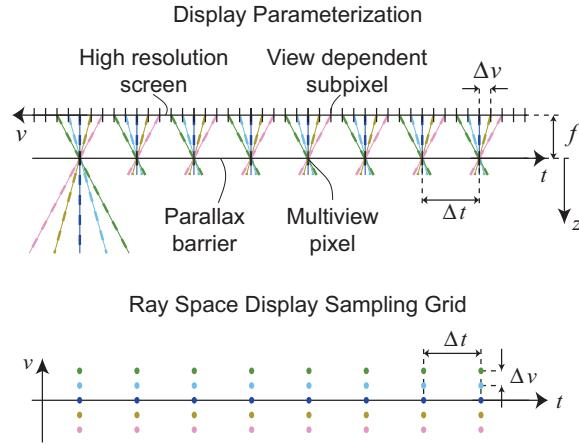
**Figure 2:** Parameterization of a scanline of a multiview display and corresponding 2D sampling grid. Because the  $v$  coordinate of a ray is relative to its  $t$  coordinate, all vertical rays (shown at the top of the figure) lie on the  $t$  axis with  $v=0$  (shown at the bottom).
