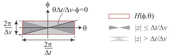
**Figure 3:** Ray-space bandwidth of automultiscopic displays. Note that the relative scaling of the  $\phi$  and  $\theta$  axes is arbitrary. We chose the scaling to indicate the relative resolution of the two axes, which is usually two orders of magnitude larger in the spatial direction ( $\theta$  axis) than in the angular direction ( $\phi$  axis). The depth of field of the display is given by the diagonals of its rectangular bandwidth.
