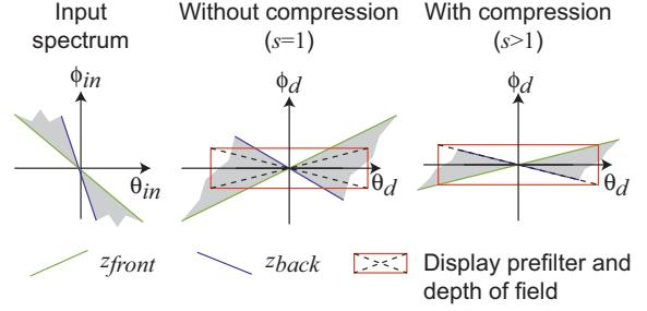
**Figure 8:** Visualization of depth compression: input spectrum (left), spectrum mapped to display coordinates without depth compression (middle), spectrum mapped to display coordinates such that a given scene depth range is in focus (right).
