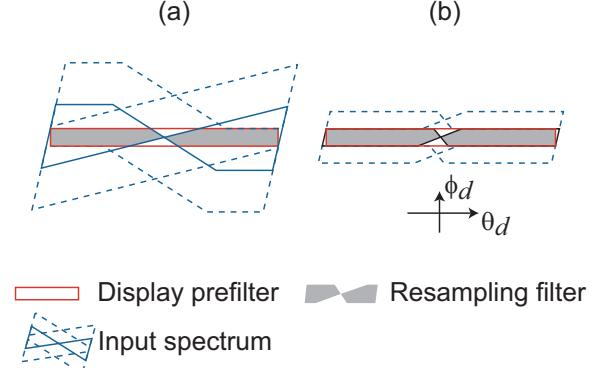
**Figure 10:** Illustration of minimum sampling using display coordinates. (a) Minimum sampling of a given scene by packing replicas of the input signal as tightly as possible. (b) Increasing the camera aperture allows for tighter packing and reduces the number of required cameras.
