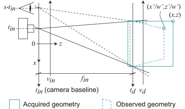
**Figure 7:** To change the size of the baseline, we scale rays along  $t_{in}$  while preserving their intersection with  $t_d$ .
