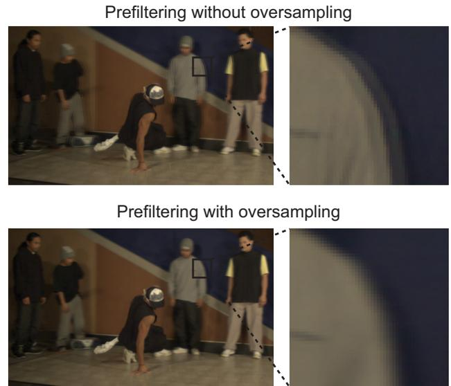
Figure 5: Comparison of pre-filtering with and without oversampling. Prefiltering without oversampling leads to aliasing problems appearing as ghosting artifacts, shown at the top. Oversampling avoids these problems as shown at the bottom.
