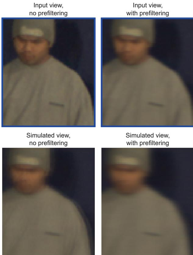
**Figure 6: Comparison of simulated display views with and without pre-filtering.** At the top, we show an input view with and without prefiltering. At the bottom, we show simulated views of the display as seen from a single eye. Ghosting artifacts appear if we omit pre-filtering, as shown on the left. The simulated view with pre-filtering, on the right, has a shallow depth of field, but it does not show any artifacts.
