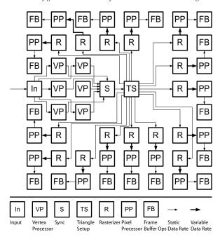
**Figure 1:** Reference pipeline layout on an 8 × 8 Raw configuration. Squares represent Raw tiles. Data arrives from an I/O port off the edge of the chip, and data is written to off-chip memory by tiles assigned to frame buffer operations. Unallocated tiles have been removed to clarify the routing.
