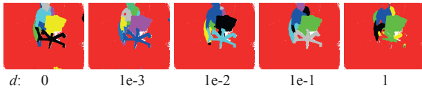
Figure 10: Setting the bias d (dataterm) to zero leads to artifacts in difficult regions (close to the boundary, behind the person’s head), as motions are favored which explain the points as being occluded as often as possible. These artifacts are fixed with a small bias. Large values will break the method, as free-space violation becomes cheaper than occlusion.
